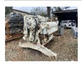
MTU USA BUILT MTU DDC V16 DIESEL ENGINE, PART NO. 5260900014 INCLUDES STARTER & ALTERNATOR, MTU AUSTRALIA REBUILD REBUILD DATE: 9/9/2011 S/NO: 5272003150 RATED: 2500HP
