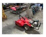
1 ROTARY HOE/POWER TILLER, SPLENDOR MOD: BK-56BL1 POWERED BY LONCIN PETROL ENGINE, 196cc 4 x BLADE, 480mm (W), 350m (DEPTH)
