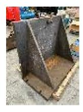
1 ENGINEERING ANGLE BLOCK, 1300 x 1015 x 610mm CAST STEEL
